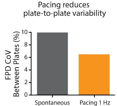
Pacing Pluricyte® Cardiomyocytes with the E-Stim+ Classic MEA plate significantly reduces well-to-well variability in field potential duration (FPD) ( $p=0.01$ ) as well as variability between plates. Variability was measured as the coefficient of variation (CoV) across wells (left) and across plates (right).
