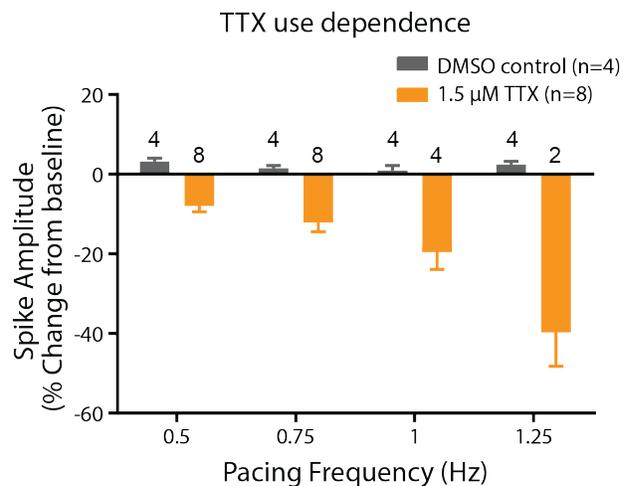
(Left) Reverse use dependence of E-4031, a HERG potassium channel blocker, revealed by pacing Pluricyte® Cardiomyocytes on the E-Stim+ Classic MEA 48 plate. (Right) Use dependence of TTX, a sodium channel blocker, revealed by pacing Pluricyte® Cardiomyocytes on the E-Stim+ Classic MEA 48 plate. (Both) Bars represent mean  $\pm$  1 standard error of the mean. Numbers above the bars indicate the number of wells successfully paced.
