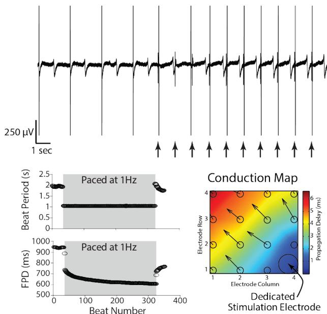
Pacing stimuli set beat rate at 1Hz (top, arrows). Beat period and field potential duration quickly adapt (bottom left). AxIS quantifies key parameters, such as conduction, with real-time visualization (bottom right).
