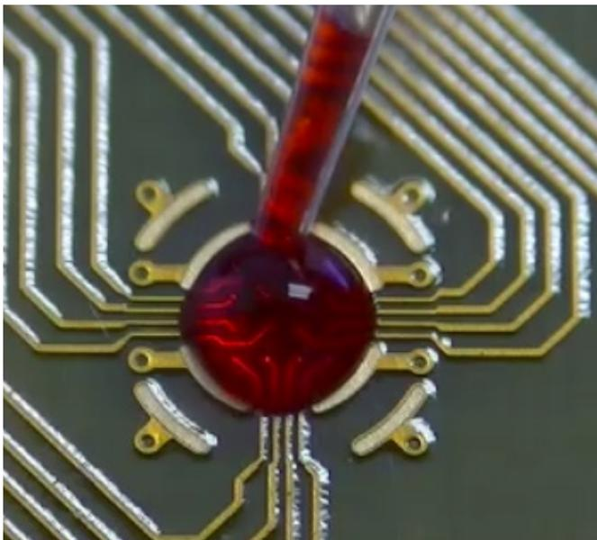
**Base of the AccuSpot Classic MEA 48 plate with the wells removed. On-plate spotting guides (patent pending) center the droplet over the recording electrode array, increasing plate preparation speed and accuracy.**
