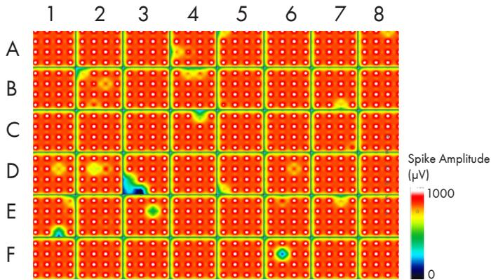
**Activity Map illustrating excellent recorded activity across the AccuSpot Classic MEA 48 plate (16 electrodes per well). Data shown is the Depolarization Spike Amplitude from iCell<sup>2</sup> CMs (Cellular Dynamics International) at day 7 post-thaw.**
