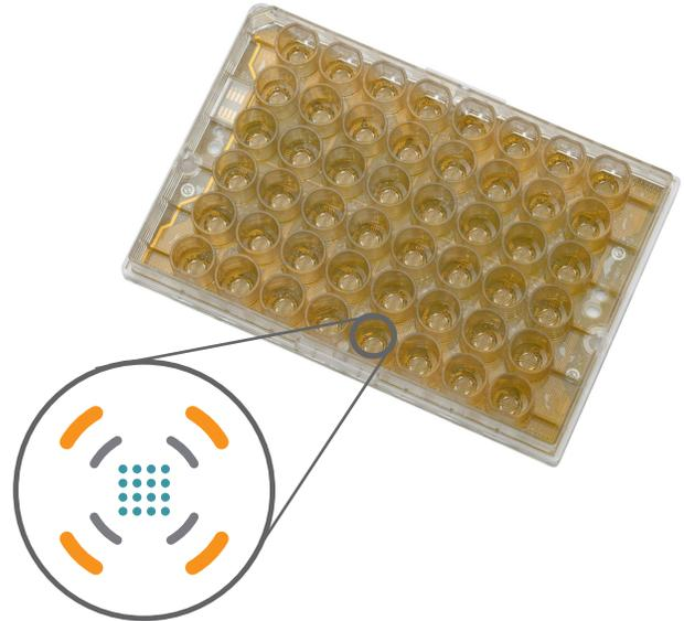
**AccuSpot™ Classic MEA 48 plate (M768-KAP-48A) for the Maestro MEA systems. Inset: Schematic of single well illustrating the AccuSpot on-plate spotting guides (gray), recording electrodes (blue), and grounds (orange).**
