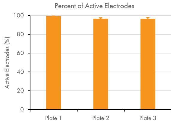
**Percent of active electrodes across 3 AccuSpot Classic MEA 48 plates. Displayed are the mean  $\pm$  standard error across all 48 wells on each plate (16 electrodes per well, 768 electrodes per plate).**
