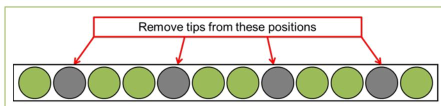
**Figure 2: Tip Loading Strategy for a 12-channel Pipettor**
