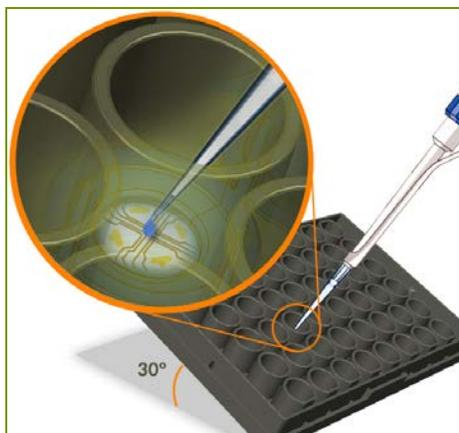
**Figure 1: Droplet Placement**
