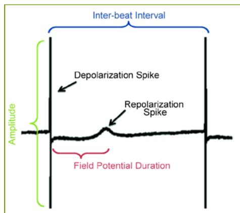
**Figure 3: MEA Cardiac Field Potential and Analysis Parameters**
