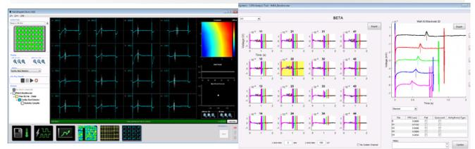
Axion's Maestro MEA systems (top) integrate seamlessly with AxIS software (bottom left) to provide cardiac beat, FPD, and conduction tracking. The CiPA Analysis Tool (bottom right) enables semi-automated FPD detection and arrhythmia classification across files.
