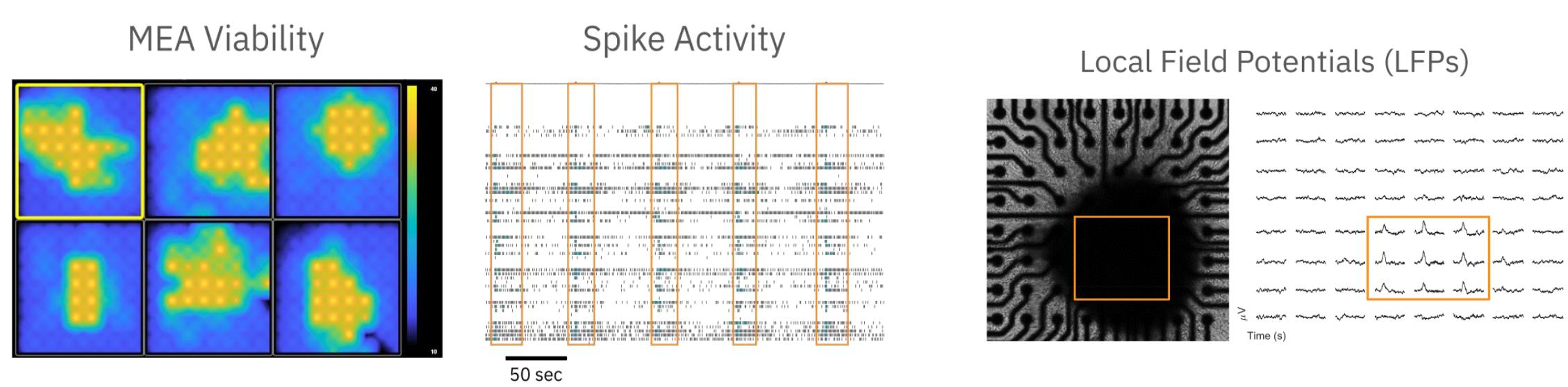
The Maestro MEA platform can be used to characterize the activity of iPSC-derived neural organoids in real-time by measuring important neural metrics such as viability, neural spike activity, and local field potentials (LFP).
