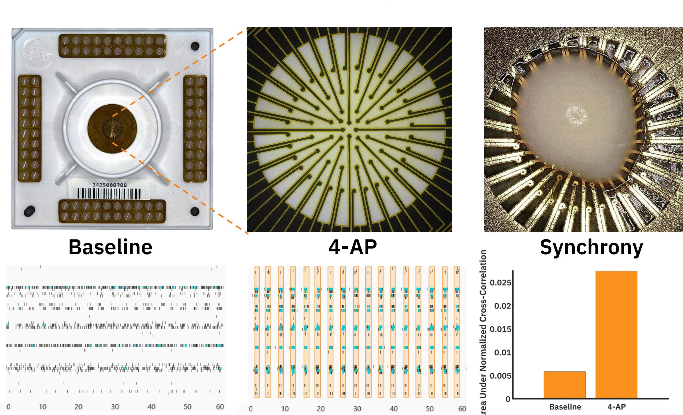
The 3DMap™ MEA uses flexible cantilevers with 64 electrodes that bend to conform to plated neural organoids, enabling 3D electrophysiological recording. Activity was measured from a pre-made midbrain organoid (STEMCELL Technologies, Cat. # 200-0793) at 111 days post differentiation. The organoid was also dosed with 4-AP, which led to marked increases in network bursting and synchrony.
