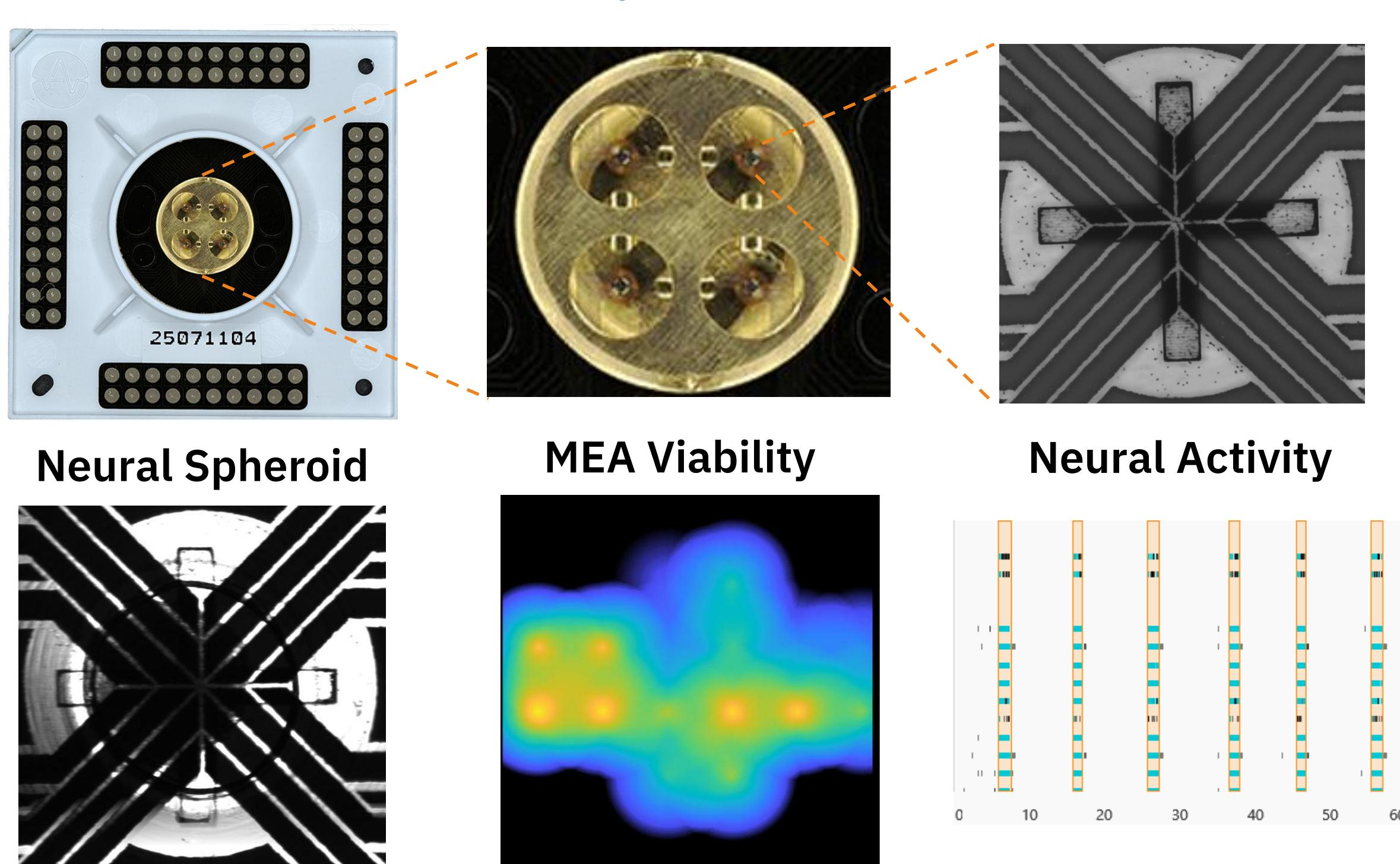
The SpheroHD MEA is comprised of an Ibidi 4 Well Fultrac micro-insert adhered to a microelectrode array chip, with each microwell positioned over an array of 16 high-density (50  $\mu$ m spacing) electrodes. The chip's design leads to improved plating accuracy, ensuring the capture of neural activity on several electrodes even when measuring from small spheroids.
