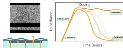
The impedance is measured from electrodes embedded in the bottom of each well. As cells cover more of the electrode, impedance increases in proportion to the number of viable cells. If a perturbation kills the attached cells, impedance decreases as the cells lyse.
