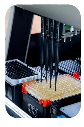
The 4-channel pipet head supplies flexibility for 48- and 96-well MEA plates, and the requisite precision for critical steps in plate preparation.
