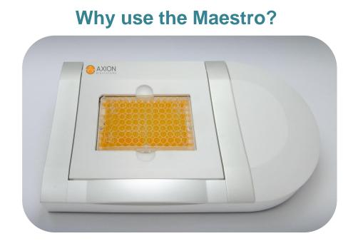
Axion's Maestro multiwell microelectrode array (MEA) platform enables high throughput evaluation of neural and cardiac activity on the benchtop, with an industry leading 768 electrodes across all plate formats.
