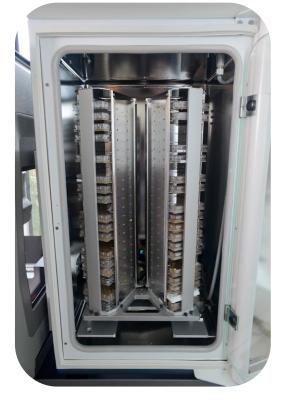
An integrated 44-plate incubator provides ample storage for high throughput MEA experimentation.
