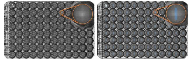
Figure 2: (A) a high-resolution scan of the 96-well plate in the Axion Portal. The insert shows well B8, directly after wound formation using the Autoscratch™ Wound Making Tool. (B) Overlay of the wound area of the scan in A. The wound area (blue) was determined using the integrated Scratch Assay software. The detected wound area of well B8 is shown in the insert.
